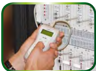
programmed and set locally with the SPI-300 programming unit from IKUSI
